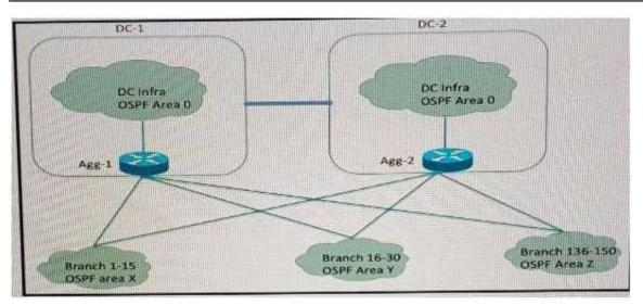
company xyz has 150 branch location across the U.S. Each branch is connected to two aggregation router one router in each data center The network is configured with Multiple OSPF with multiple OSPF areas and the aggregation router are ABRs A requirement is to keep an optimal path to the data centers and at the same time reduce the LSA propagation and SPF recomputation during a change in any part of the network Which design elements should be included on the aggregation router?
