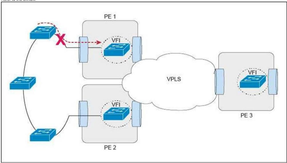
This Layer 2 ring has 10 VLANs with 1000 MAC addresses in each VLAN. Which protocol or mechanism provides the shortest traffic outage if the link marked with "X" fails?
