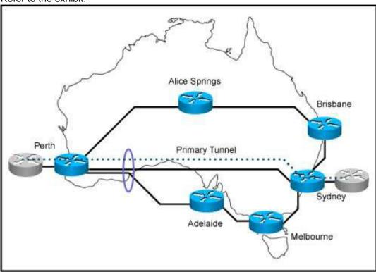
You are designing MPLS-TE for this network. The links form Perth to Sydney and from Perth to Adelaide share the same optical fiber in one given segment. Which feature should you implement to eliminate the risk that a backup tunnel is installed over the same optical fiber as the primary one?
