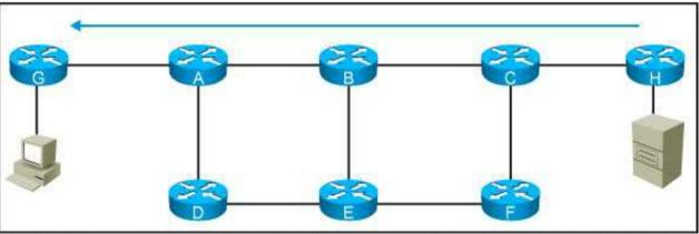
This network is running IS-IS as the single routing protocol and the LSP and SPF timers are aggressively configured so the network converges in subsecond. The customer reports that router B had a memory crash and reloaded. Which resulted in some packets from the application being lost. The application servers are behind router G and the end users are behind router H, which design change should be made to prevent this packet-loss problem from reoccurring?
