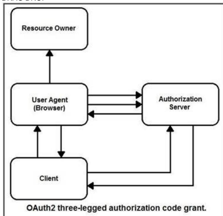
Refer to the exhibit. Drag and drop the steps from the left into the correct order of operation on the right for a successful OAuth2 three-legged authorization code grant flow.
