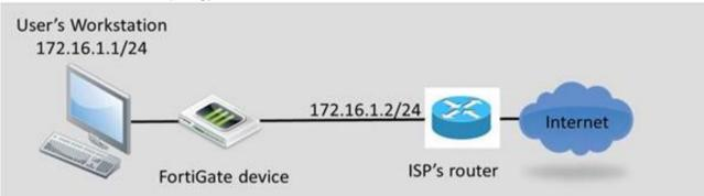
The workstation, 172.16.1.1/24, connects to port2 of the FortiGate device, and the ISP router, 172.16.1.2, connects to port1. Without changing IP addressing, which configuration changes are required to properly forward users traffic to the Internet? (Choose two)
